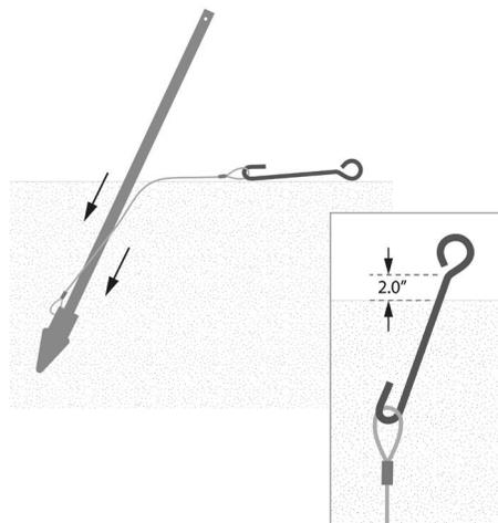
2. Drive anchor until the eye of the setting tool is 2" above ground level.
