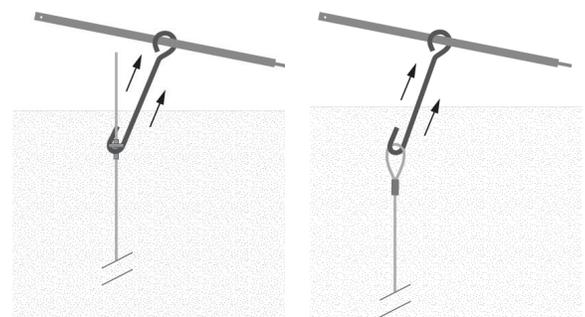
3. Use a JackJaw or drive rod to pull up and set the anchor or repair kit.
