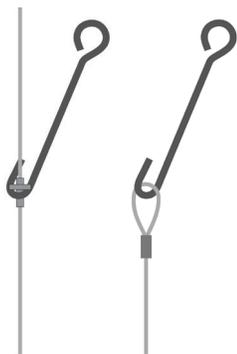
1. Position the hook around the ferrule or through the top loop of the anchor cable.
